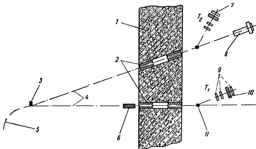
FIG. 1. Experimental Arrangement. 1 - Concrete shield; 2 - Collimators; 3 - Target (Be); 4 - Neutrons; 5 - Protons ( $E_p = 580$  mev); 6 - Sample; 7 - Telescope; 8 - Bi-Chamber; 9 - Detecting telescope; 10 - Filter; 11 - Scatterer
